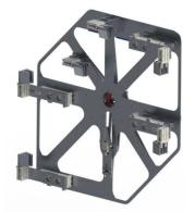
Sometimes, EoAT design requires lateral thinking. In this example, pneumatic grippers grip a rubber edging, whilst a secondary set of cylinders expand the product outwards, creating clearance to remove the product from the mould cores.
